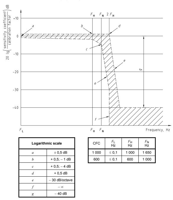
Figure 2 — Frequency response limits — CFC 1 000 and CFC 600
