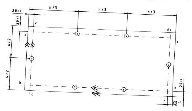
Figure 2: Measuring points and lines for door leaf
