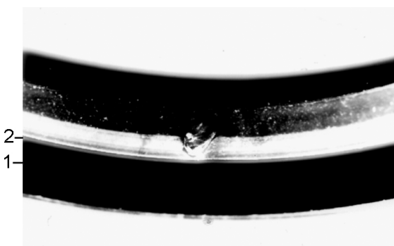
Figure 5 — Inclusion: foreign material
