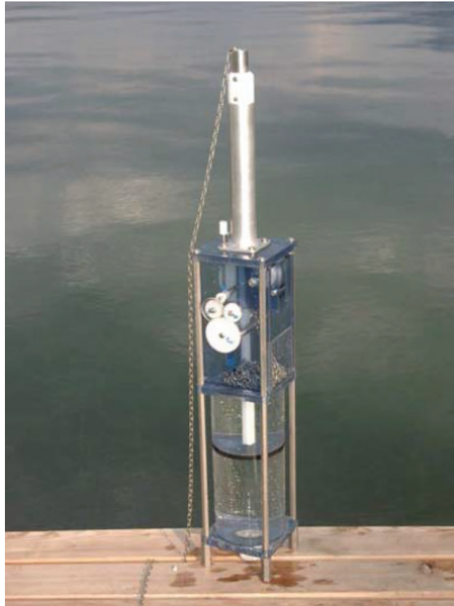
Figure A.7 — Mechanic integrating water sampler (Photo UWITEC Mondsee, Austria)
