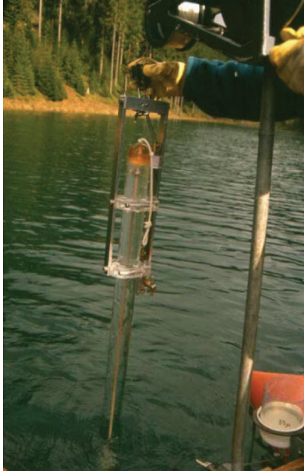
Figure A.5 — Tube integrating sampler as originally developed by Pauli
