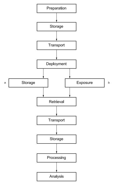
NOTE Field controls (a) are stored during the period of field exposure of deployed passive sampling devices (b).
