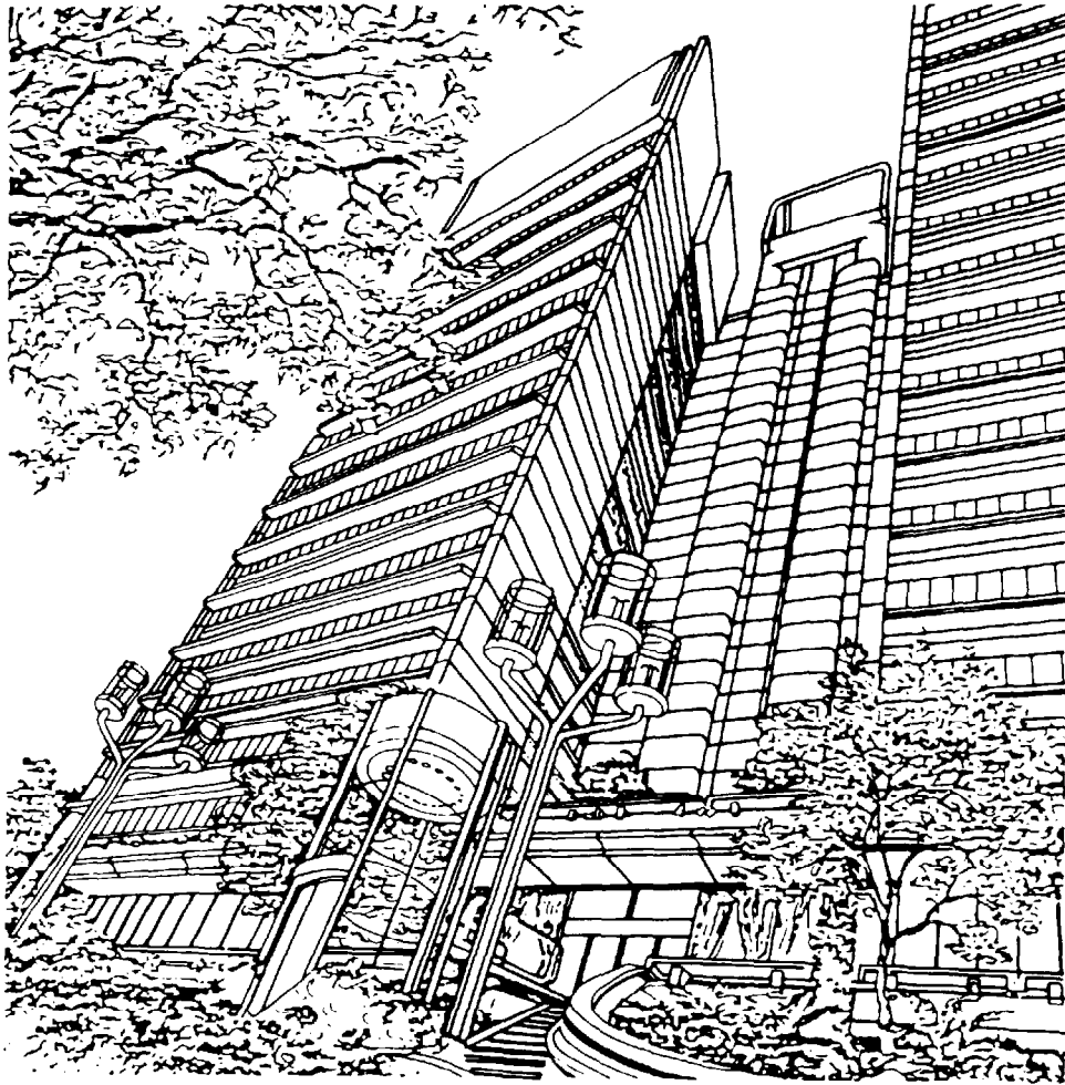
Figure A.5 — Exterior space image, projection with inclined projection plane and three vanishing points according to the method described in 7.5.1
