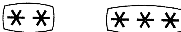
Figure 8 — Identification symbols for "three star" cabinets and "two star" sections (for further details, see figure 15)
