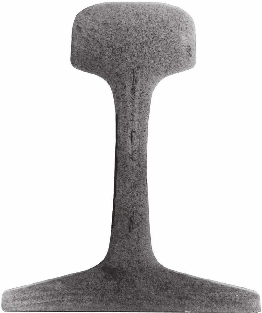
Figure H.6 — Central web streaking extending into the head or base
