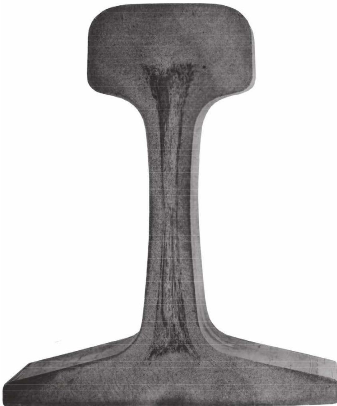
Figure H.13 — Inverse or negative segregation >6 mm wide, extending more than 13 mm into the head or base
