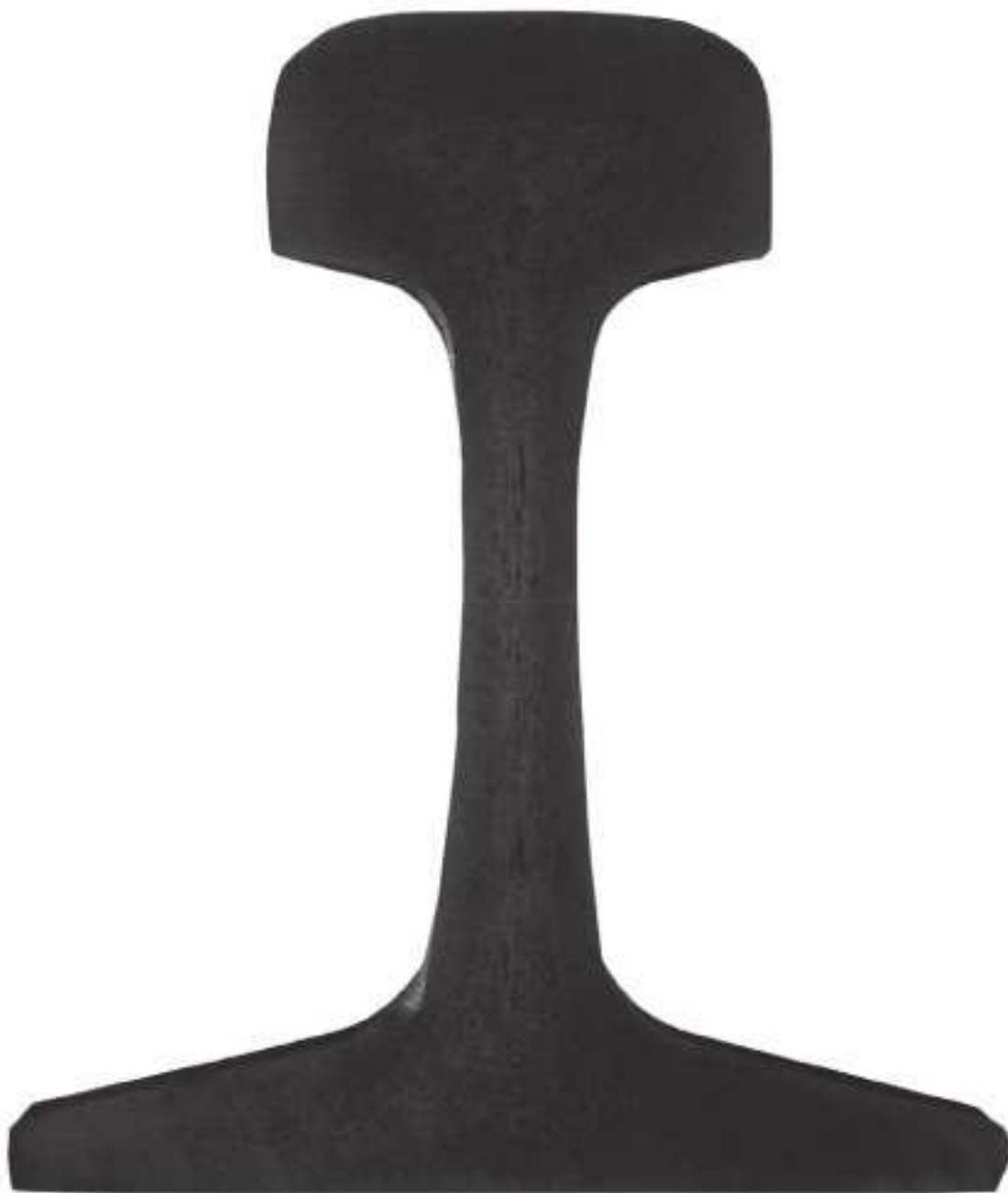
Figure H.11 — Scattered segregation extending more than 25 mm into the head or base
