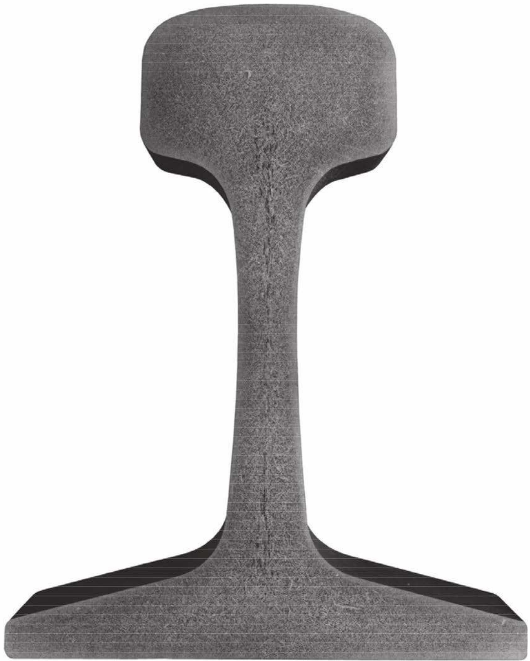
Figure H.10 — Scattered central web streaking from the web into the head and base
