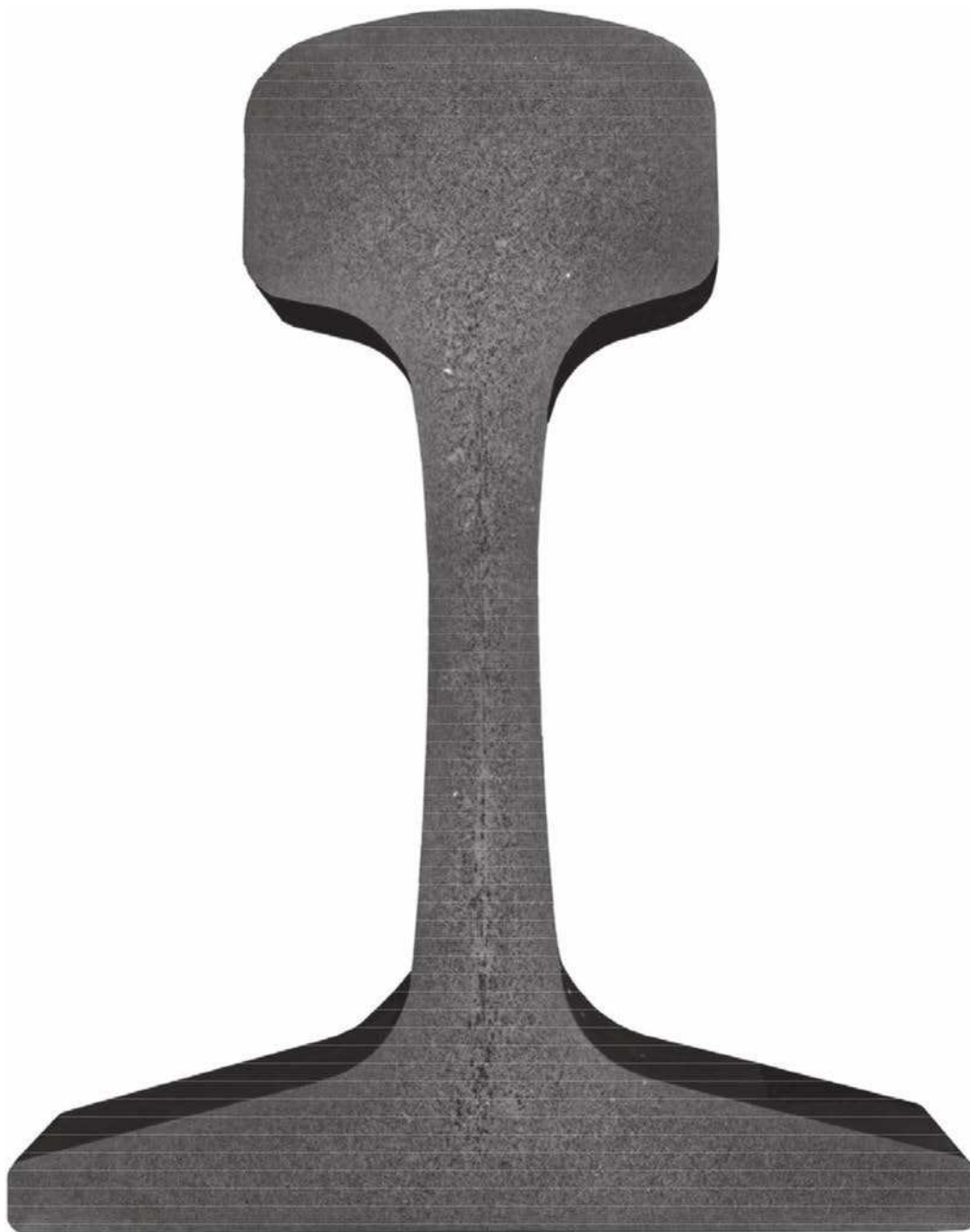
Figure H.7 — Central web streaking extending into the head or base
