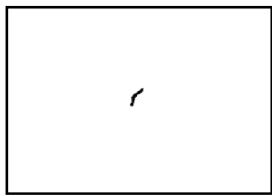
a) Maximum size allowed for a non-relevant indication for severity level LP 3c
