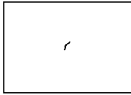
a) Maximum size allowed for a non-relevant indication for severity level LP 3a
