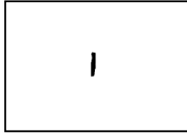
a) Maximum size allowed for a non-relevant indication for severity level LM 5a or AM 5a
