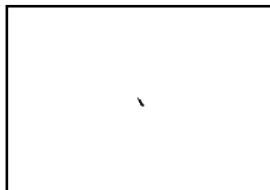
a) Maximum size allowed for a non-relevant indication for severity level LM 1a or AM 1a
