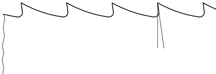
Figure 9 — Positive skip tooth Figure 9 — Denture évidée positive
