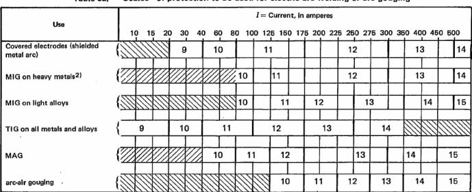
Table 5a) — Scales<sup>1)</sup> of protection to be used for electric arc welding or arc gouging
