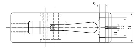
NOTE The lower part of the grip is spring loaded with a spring tension of between 5 N and 15 N to minimize deformation of the rubber.
