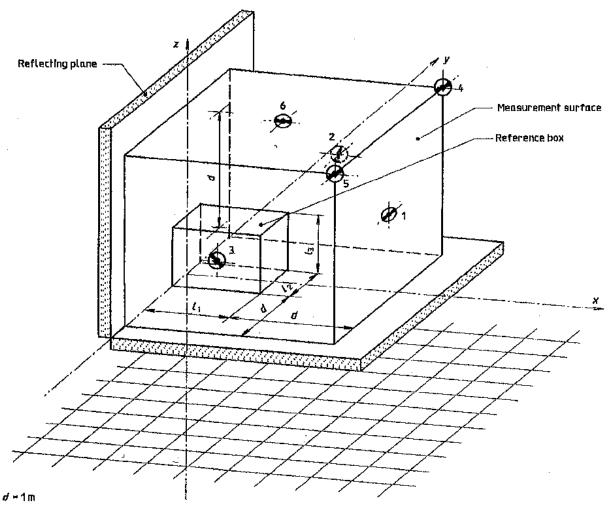
NOTE – This form of array is based upon the microphone array described in ISO 3744:1981, annex C.
