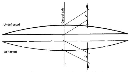
a and b are medial deviations before and after deflection a+b is medial deflection
