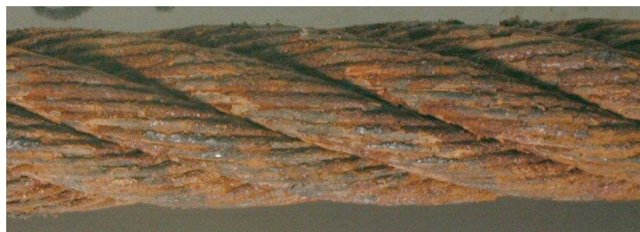
Figure H.3 — Surface of wire now greatly affected by oxidation — Rating: 60 % towards discard
