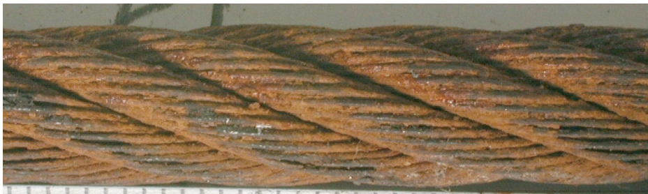
Figure H.4 — Surface heavily pitted and wires quite slack, gaps between wires — Discard immediately
