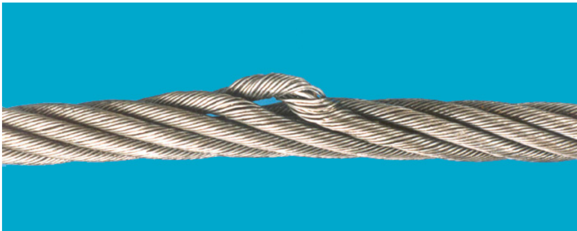
Figure B.4 — Strand protrusion or distortion
