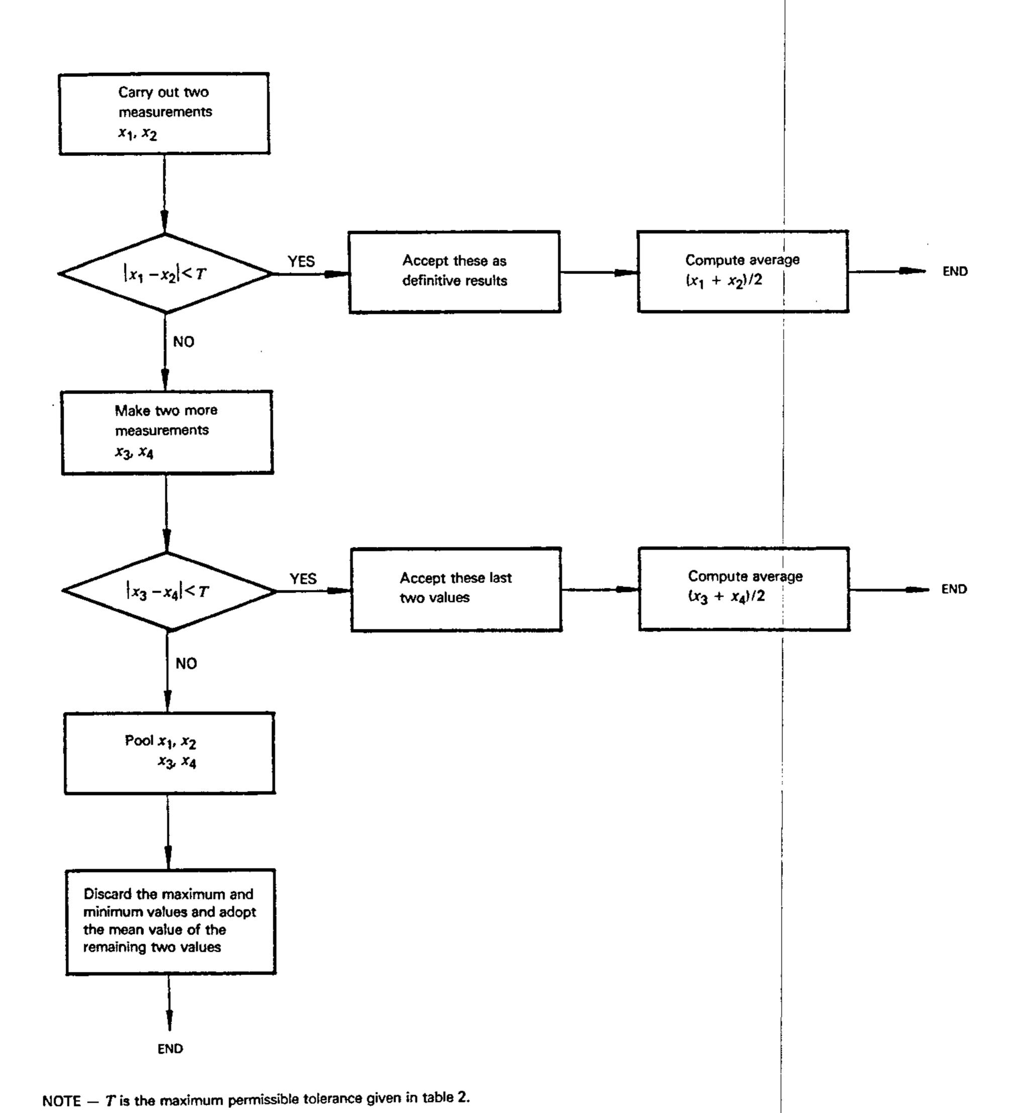
Figure 1 - Flow chart - Procedures for processing the results of moisture determinations
