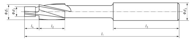
NOTE This Figure shows a counterbore with cutting diameter  $d_1$  greater than 5 mm.
