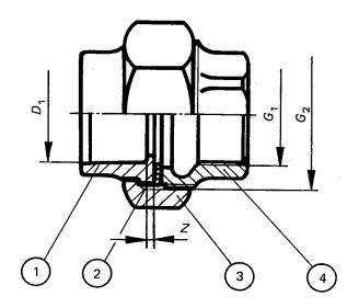
5.2 Type II — PVC/metal union (equal) with male pipe thread in metal part
