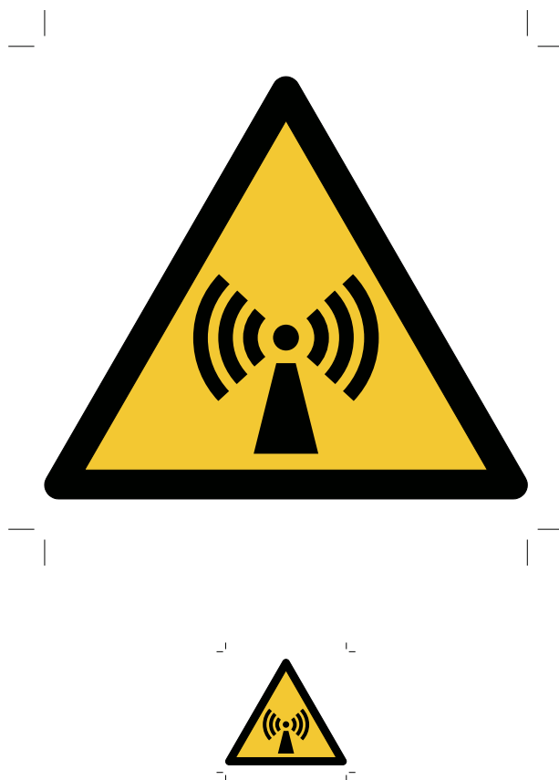
Figure 13 — Warning; Non-ionizing radiation (ISO 7010-W005) — Original size (70 mm) and size reduction to 25 %
