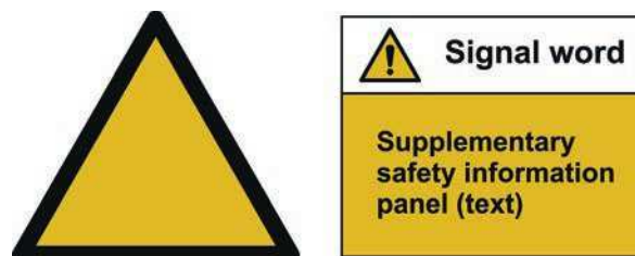
Figure 3 — Layout of safety sign with a separated supplementary safety information text panel which includes a hazard severity panel with optional signal word
