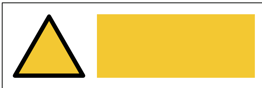
Figure 8 — Layout for a combination sign with the supplementary sign below the safety sign
