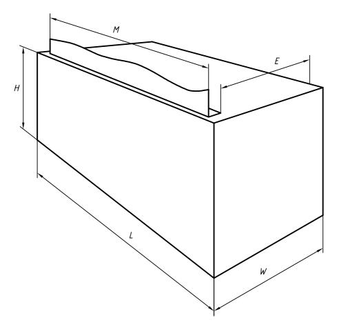
Dimension W shall never be less than dimension E on any single cassette. Dimension M is the width of the sensitized material given in Tables 1 and 2.
