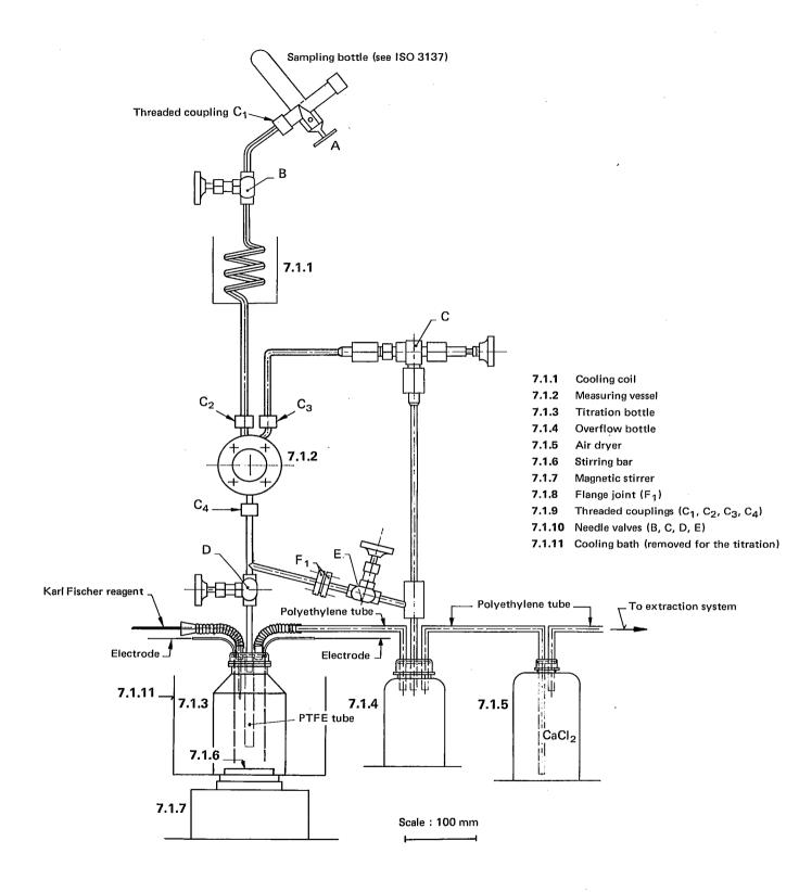
FIGURE 1 - Apparatus for measurement of the test portion and titration (7.1)
