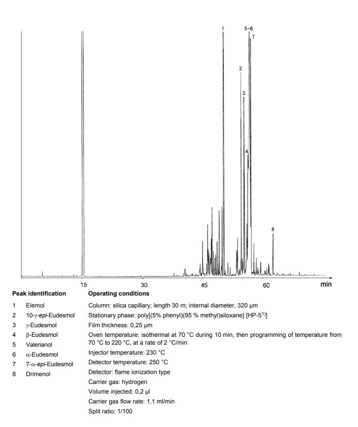
Figure A.1 — Typical chromatogram taken on an apolar column
