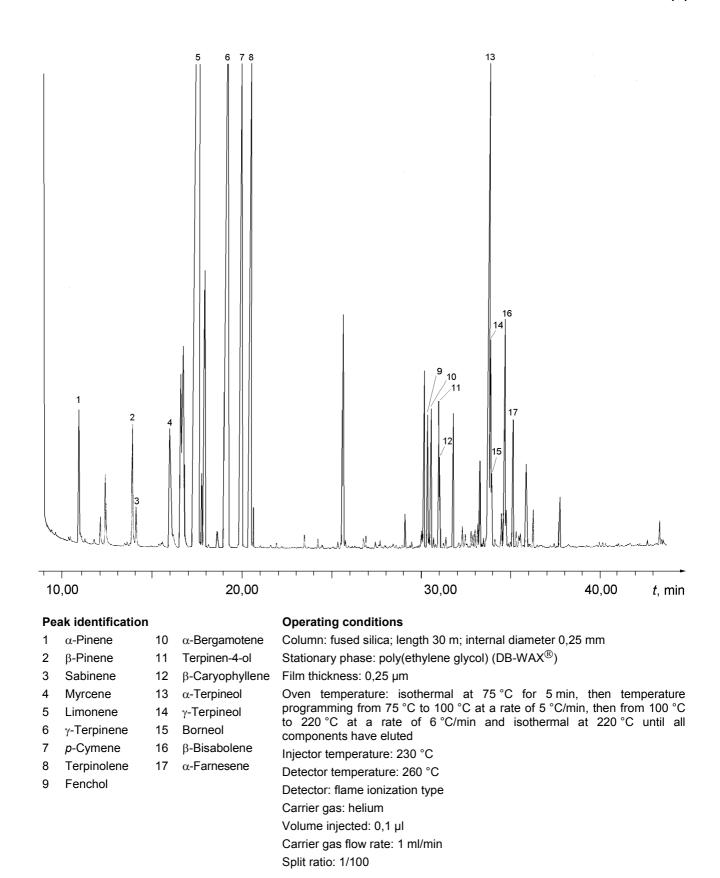
Figure A.2 — Typical chromatogram taken on a polar column
