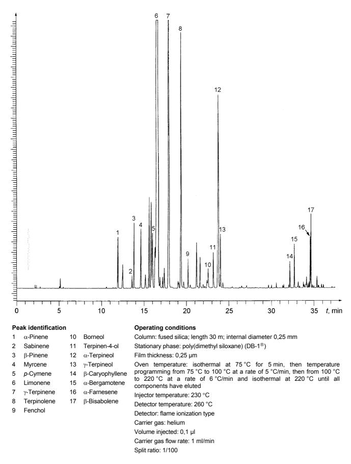
Figure A.1 — Typical chromatogram taken on an apolar column
