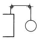
6.2.5 Tank gauge-float type, top-mounted
