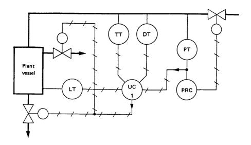
In a more complicated installation or one which does not lend itself to such a layout, the symbol for the combining controller may be repeated at each instrument and correcting unit symbol, being connected to the usual symbol for these elements by a thin line. With this type of presentation, explanatory notes, which may or may not be on the flow sheet, are essential.
