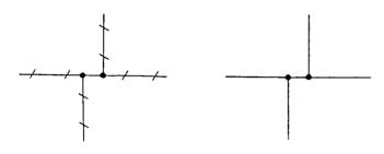
The diameter of the connecting dot shall be approximately five times the width of the associated lines.
