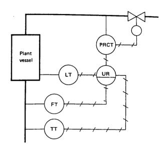
In a more complicated installation or one which does not lend itself to such a layout, the symbol for the multivariable data receiving device may be repeated at each associated instrument symbol, being connected to the usual symbol by a thin line. With this type of presentation, explanatory notes, which may or may not be on the flow sheet, are essential; for example, PRC in the following diagram denotes an instrument which does not have a transmitting function.
