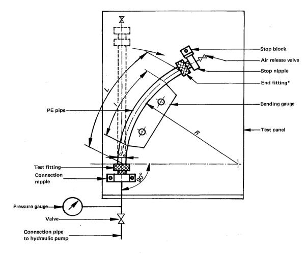
\* The end fitting is only used for closing the test specimen.
