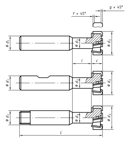
NOTE Chamfers f and g may be replaced by radii of the same value. These are optional configurations.
