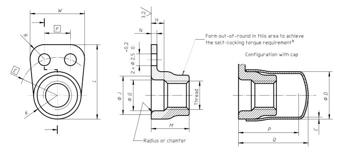
Tolerances of form and position shall conform to those specified in ISO 8788. Details of form not stated are at the manufacturer's discretion.
