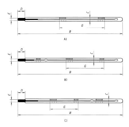
NOTE — The difference in the designs rests mainly in the position of the ice point scale. In design A, the ice point is within the scale range, in design B, the ice point is below the scale range and in design C, the ice point is above the scale range. See table B.1 for definition of letter symbols.
