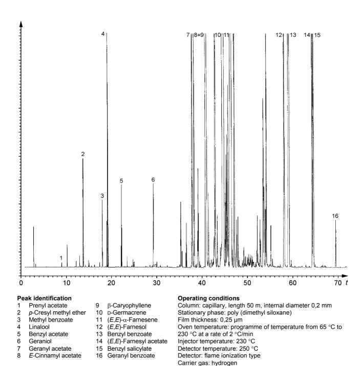
Figure A.3 — Typical chromatogram of oil of ylang-ylang "Third" Madagascar taken on an apolar column
