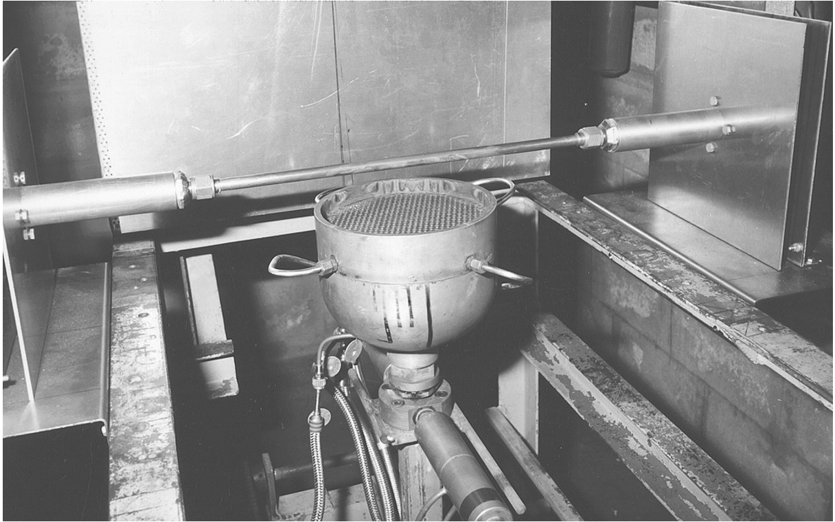
Figure A.4 — Gas burner
