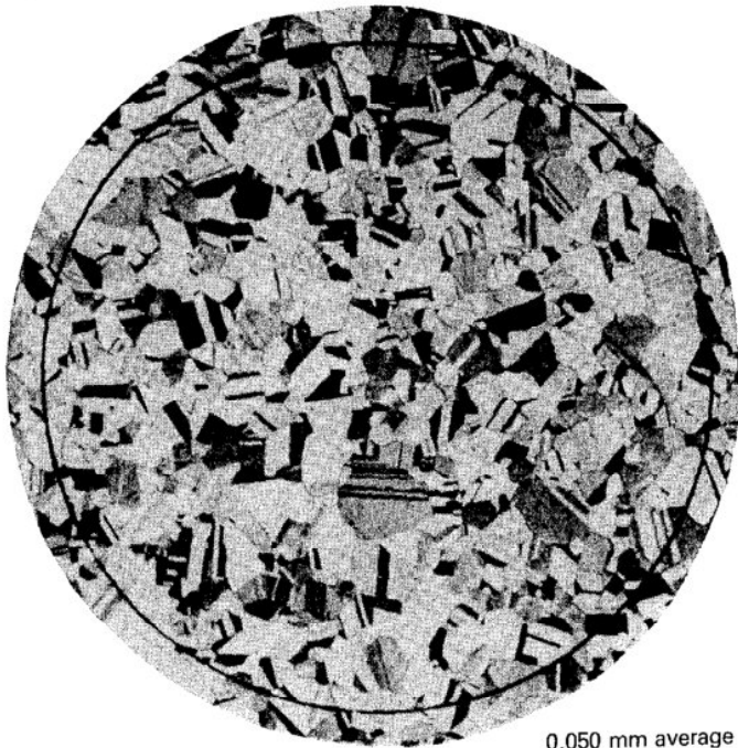
0,050 mm average grain diameter
