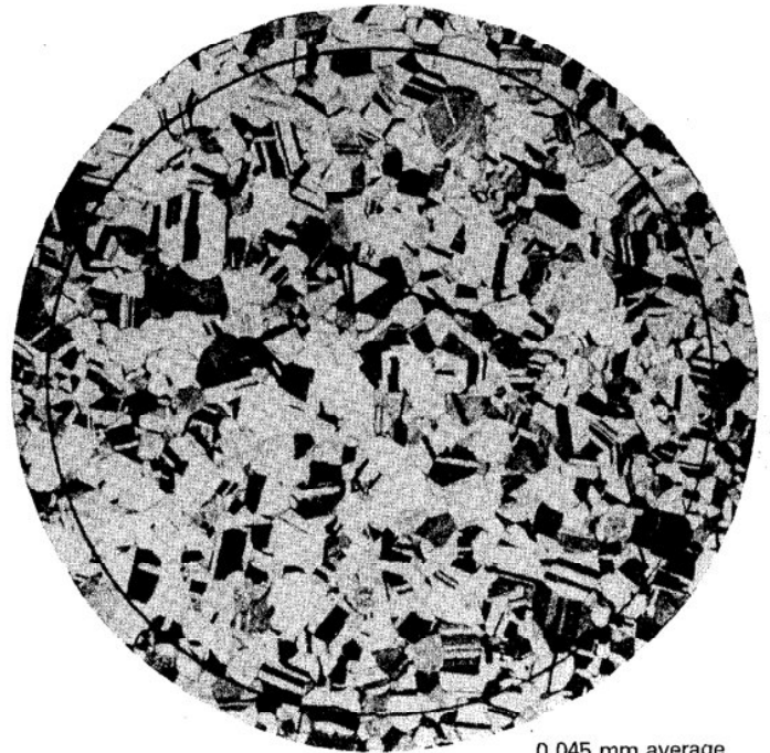
0,045 mm average grain diameter
