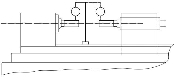
**Tolerance** Measured deviation 0,02
