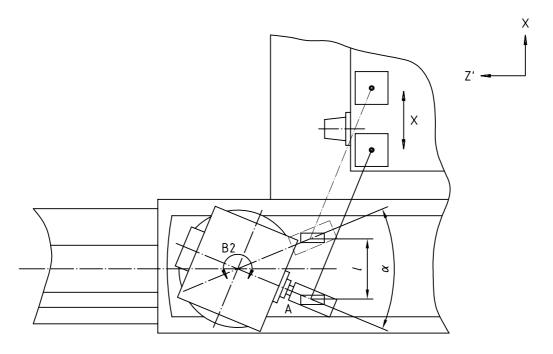
Measured deviation **Tolerance** 0.02 for l = 200
