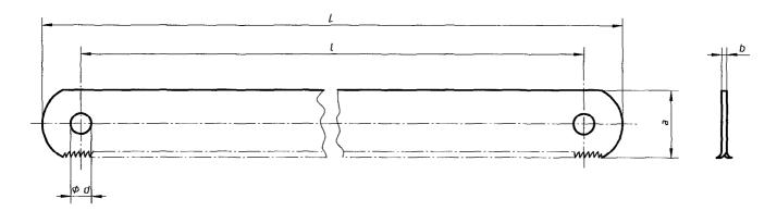
$\operatorname{NOTE}$  — The shape of the blade ends is left to the manufacturer's discretion
