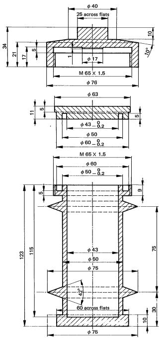
FIGURE — Suitable autoclave for the preparation of an aqueous solution of silicates not easily soluble
