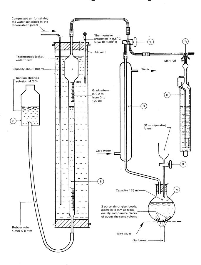
FIGURE - Apparatus for gas-volumetric determination of carbonates content
