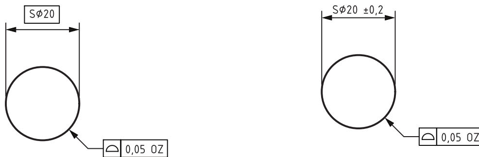
a) Surface profile specification for a sphere of defined nominal size, given by a TED with OZ indication b) Surface profile specification for a sphere of undefined nominal size with OZ indication
