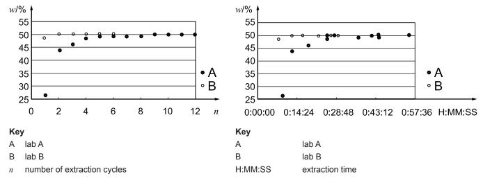
Figure C.1 — Number of extraction cycles for EPDM in 2-butanone
