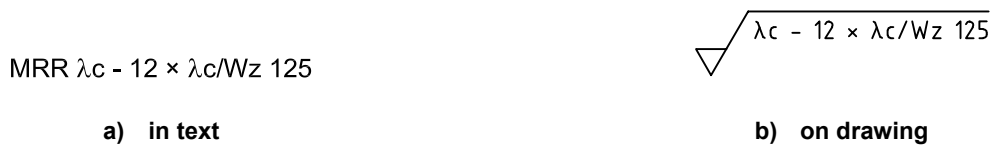
Figure 10 — Transmission band for waviness based on default cut-off \lambda_c for surface roughness
