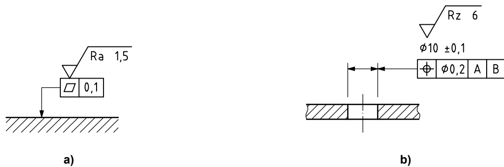
Figure 20 — Surface texture requirement — Geometrical tolerances indication
