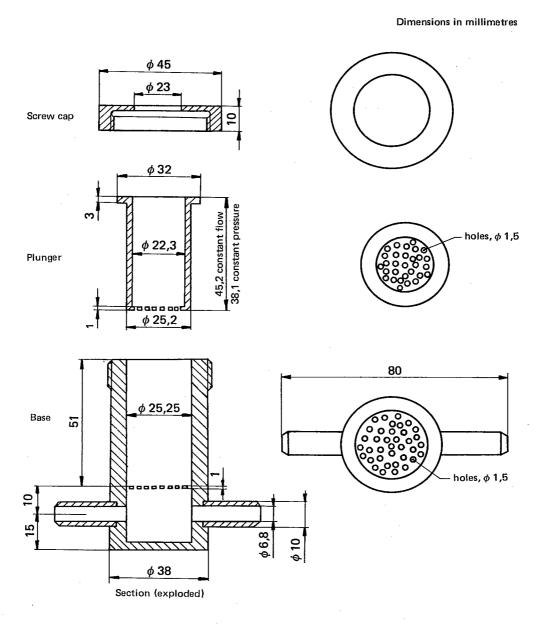
FIGURE 2 — Suggested dimensions of constant volume chamber (A) Important dimensions are 22,3 — 25,2 — 25,25 — 42,5 and 38,1 mm
