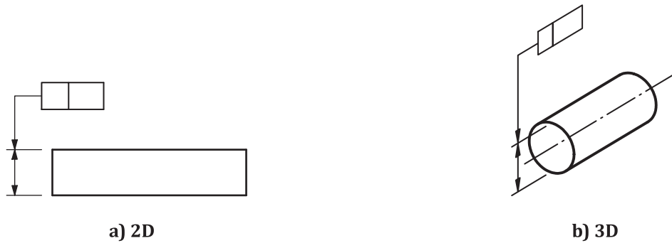
Figure 4 — Indication of derived feature specification
