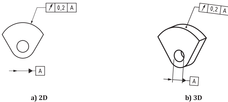
Figure 176 — Circular run-out indication
