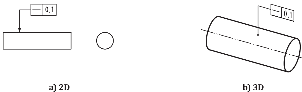
Figure 92 — Straightness indication
