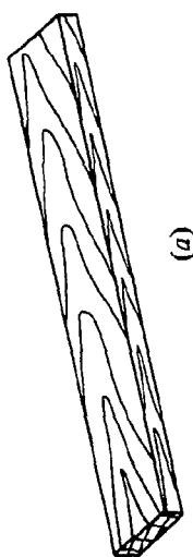
FIG. 1 — Square-edged sawn timber with parallel edges: (a) without wane (b) with wane
