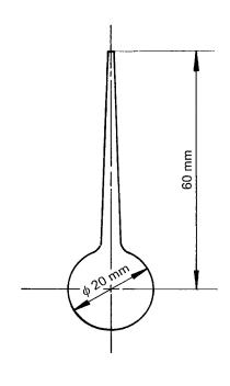
FIGURE - Spherical glass ampoule
