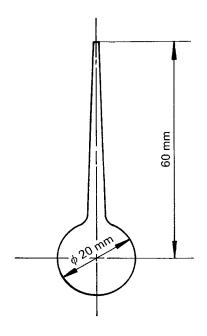
FIGURE - Spherical glass ampoule
