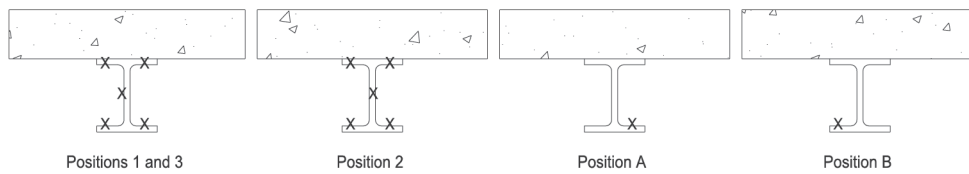
Thermocouple locations applicable to loaded 'I' and 'H' beams (17 total)
