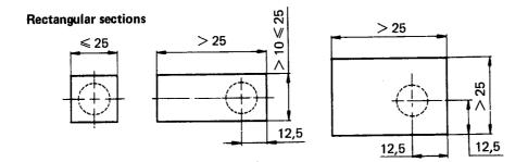
$\label{eq:figure} \textit{Figure 1} - \textit{Location of the test pieces in bars and wire}$
