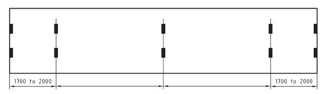
NOTE 1 Minimum requirements: 5 pairs of load transfer areas (1 pair at each end plus 3 intermediate pairs)
