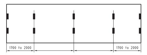
NOTE 1 Minimum requirements: 5 pairs of load transfer areas (1 pair at each end plus 3 intermediate pairs)
