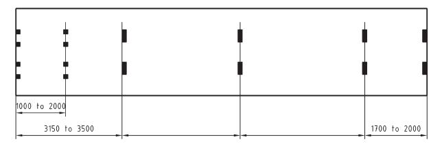
NOTE 1 Minimum requirements: 6 pairs of load transfer areas (1 pair at each end plus 4 intermediate pairs).
